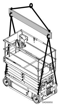
The machine may also be lifted using a spreader bar and four equal length straps or chains capable of supporting the full gross weight of the machine. Lift only using the lifting lugs provided at the four corners of the machine.
